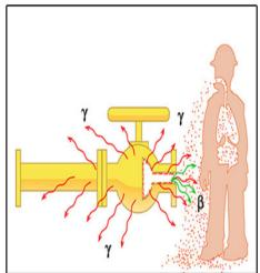
NORM stands for Naturally Occurring Radioactive Materials. NORM is all around us as background radiation, all of the time. It is part of the earth's crust and found in very low concentrations in rocks, soil and water. Background radiation emitted from NORM is small and mainly harmless; however, processes such as oil and gas production can cause NORM or TENORM (Technologically Enhanced Naturally Occurring Radioactive Materials) to build up to levels, that may be harmful to workers' health or the
